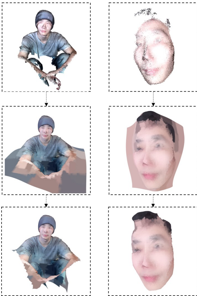
Figure 1: 3D surface reconstruction of a person (left) and a face (right). The top row are input point clouds, the middle row are reconstructed mesh using Poisson Surface Reconstruction, the bottom row are ones after cropping the redundant parts.
