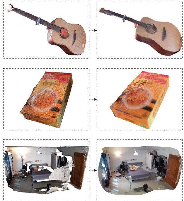
Figure 2: 3D surface reconstruction from point clouds (left column) to reconstructed surfaces (right column) of a guitar, a yellow box and a scene of bedroom.
